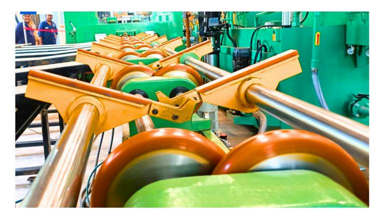
This advanced grinding equipment was capable of processing sizes ranging from 10 mm to 50 mm in diameter and set a new benchmark for precision, efficiency, and high-quality production at the plant. It also allowed the company to better meet the needs of customers, who rely on bright rod applications, such as the industries of automotive, engineering, and construction.
