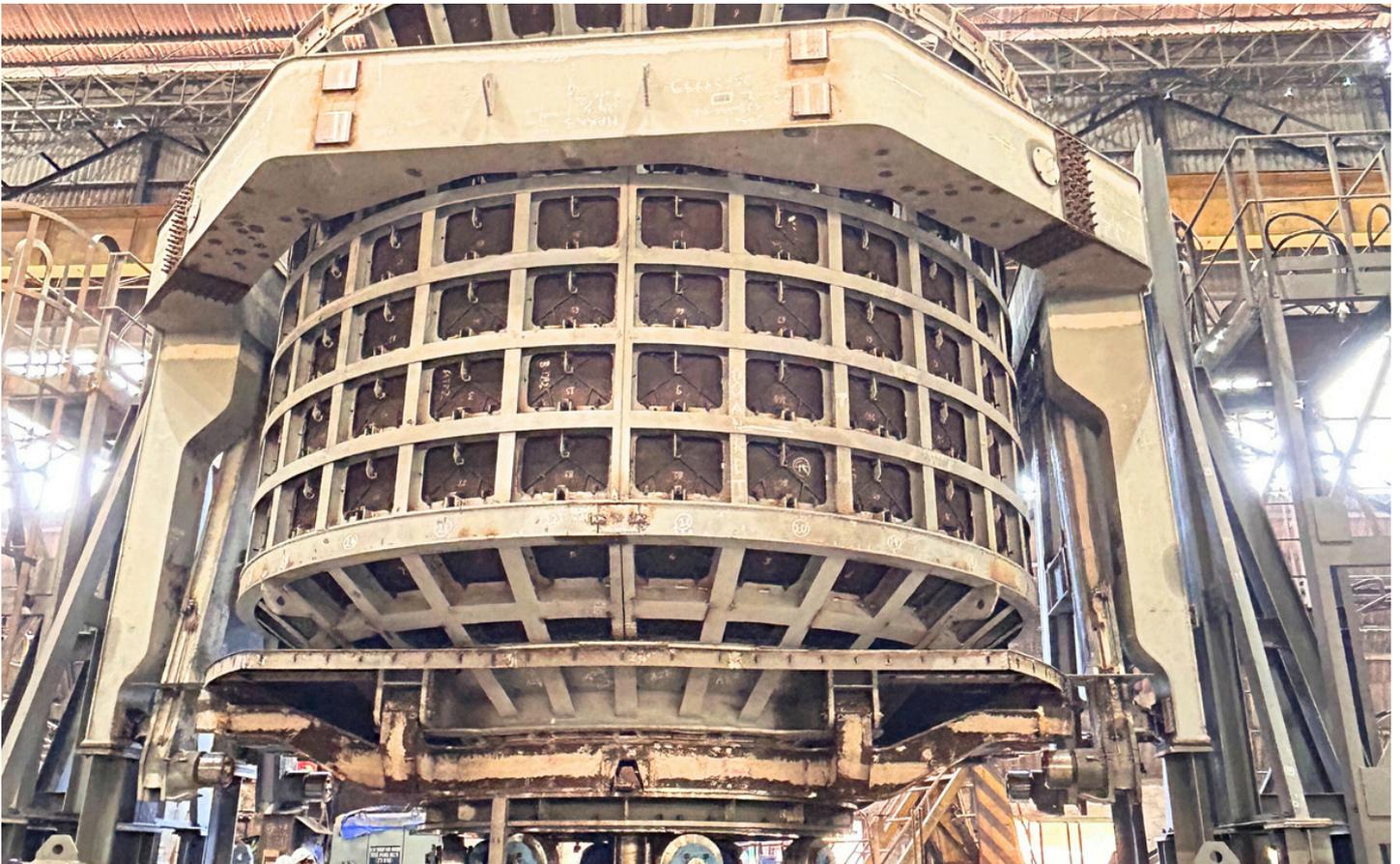
This critical component is designed for the advanced Coke Dry Quenching (CDQ) process, which replaces traditional wet quenching methods to significantly reduce CO<sub>2</sub> emissions and conserve water while enhancing coke quality in steel manufacturing. The CDQ system operates by dry cooling coke using nitrogen gas circulation, offering an environmentally friendly and energy-efficient alternative.
